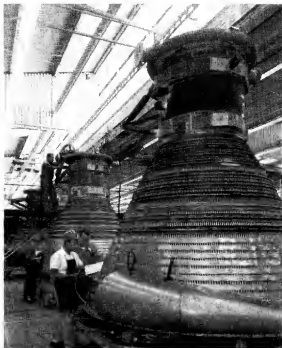
The production line for F-1 engine thrust chambers at Rocketdyne.
